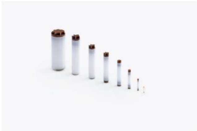
Figure 1: MAS rotors with different diameters for different spinning speeds
