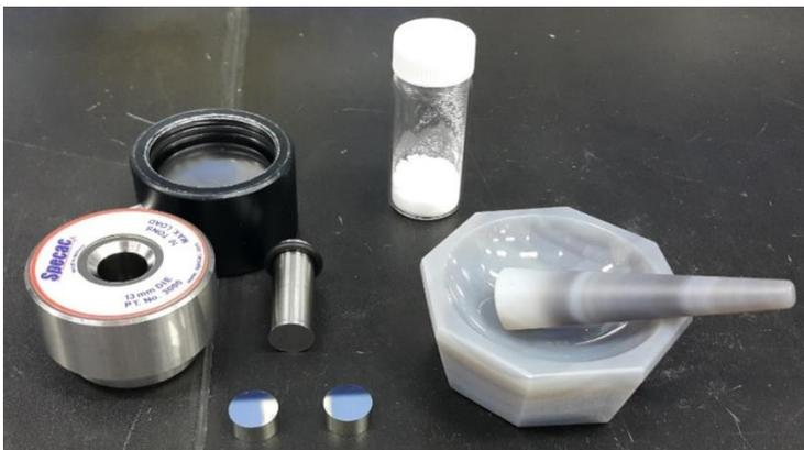
**Step 1.** The powder sample and KBr must be ground to reduce the particle size to less than 5  $\mu$ m in diameter. Otherwise, large particles scatter the infrared beam and cause a slope baseline of spectrum.
