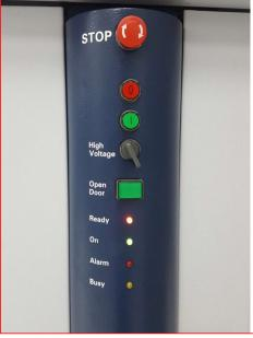
You can check machine condition through 'Status Light' located at bottom of both sides.
