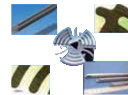
Material : SKD 11, Diameter: 70, 100 mm Roughness : 2.5 μm (Rz), Geometric tolerance : ± 3 mm Wire : 0.02 mm, Cutting liquid : Water
