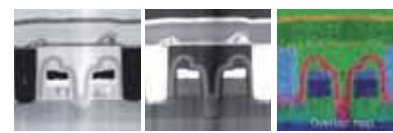
STEM HAADF Image STEM BF Image EDS Mapping [Semiconductor device]
