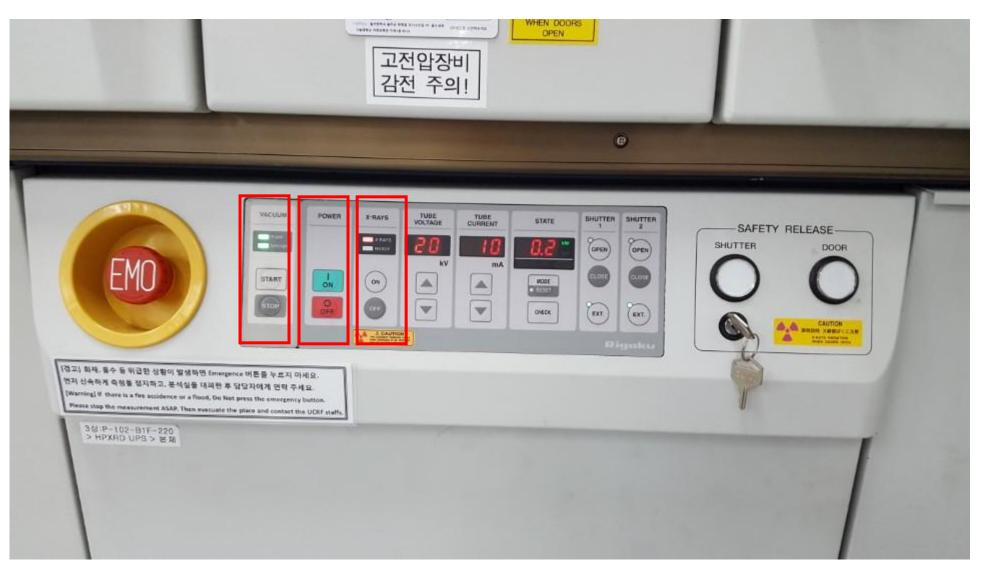
**HPXRD** is high power X-ray Diffraction machine.
