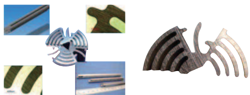
Material : SKD 11, Diameter : 70, 100 mm Roughness : 2.5 \mu\text{m} (Rz), Geometric tolerance : \pm 3 mm Wire : \Phi 0.02 mm, Cutting liquid : Water
